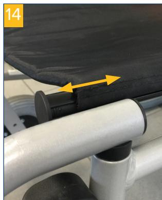
Now you can pull the frame forward to the next hole (a total of 3 times) and reinsert the screws.
