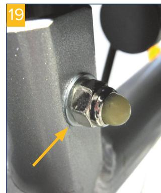
Reinsert the screws, put on the knurled nuts and tighten them.
