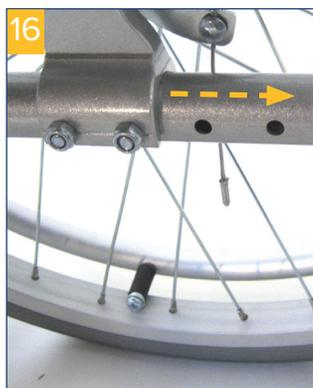
Now you can pull the frame forward to the next hole (a total of three times) and reinsert the screws.
