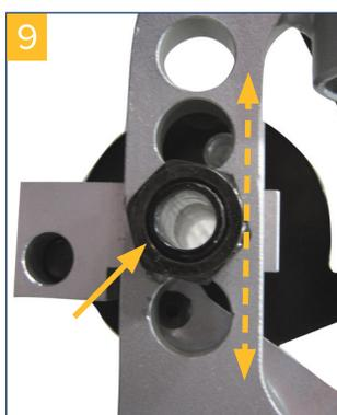
**Ensure that the wheel axle is properly tightened!**
