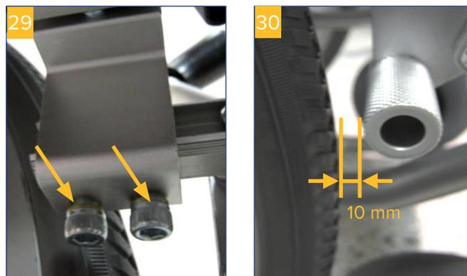
**Ensure that all screws are reinserted and tightened!**
