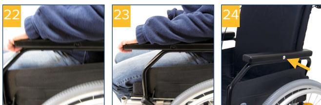
**The spring button must lock back into position after adjustment. Select the closest position, if necessary.**
