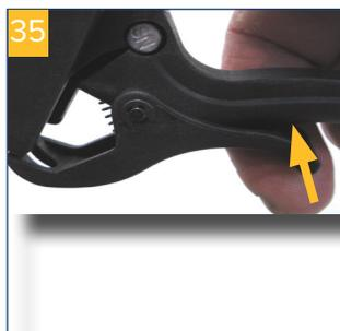
If you need to step away from the wheelchair while it is occupied, it is essential to additionally apply the parking brake.
