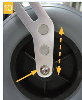
The plugs of the corresponding holes can be easily exchanged. Now move the wheel in the desired position and reinsert the wheel axle screw and tighten it (photo 10).
