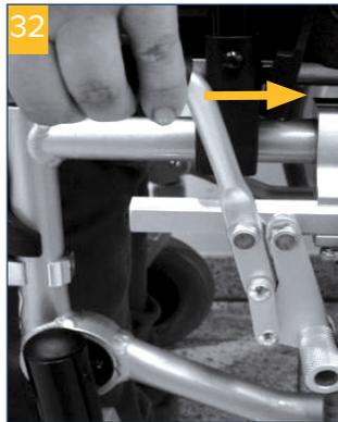
**Always ensure that the parking brake is locked by attempting to move the wheelchair.**
