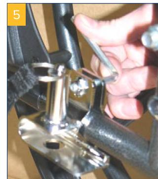
Then align the PowerStroll in the center and secure with the wing screws. When the PowerStroll is attached to the wheelchair, it should be in a horizontal position. If this is not the case, orient the power unit using the height adjustment on the PowerStroll (**photo 6**).
