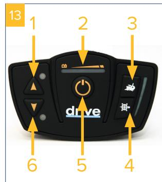
The direction of travel can be adjusted by pushing the arrow buttons (**1+6**).
