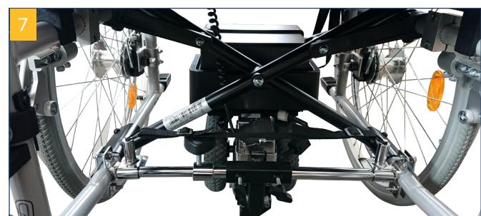
Tighten the screws so that the holders sit securely and do not rotate.
